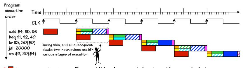
6 nS Instruction Fetch 2 n5 Instruction Decode 2 nS Register Prop Delay 5 nS ALU Operation 4 nS Branch Target 6 nS Data Access
