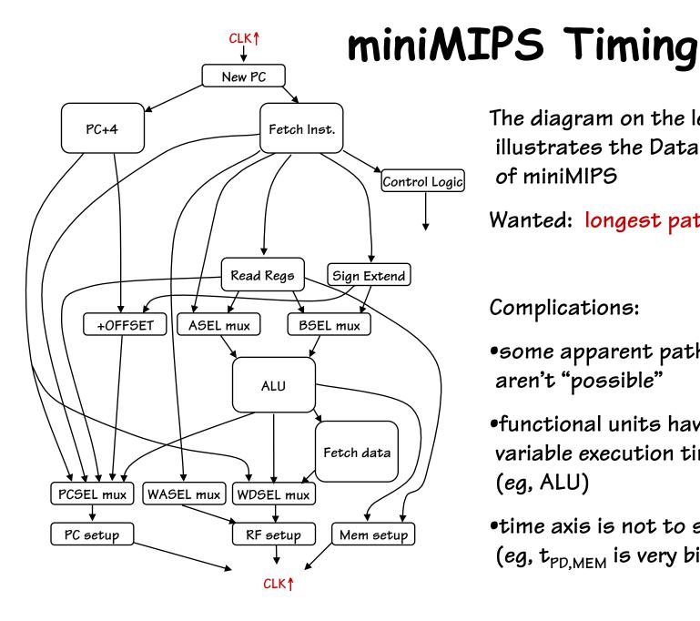
The diagram on the left illustrates the Data Flow of miniMIPS
