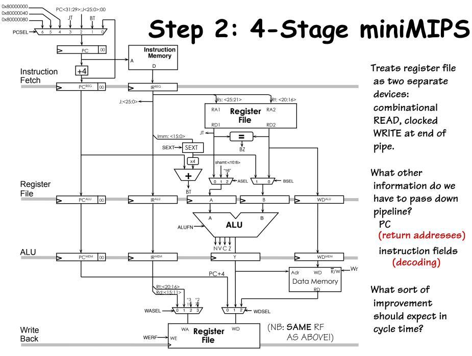
Treats register file as two separate devices: combinational READ, clocked WRITE at end of pipe.
