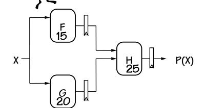
Now F & G can be working on input  $X_{i+1}$ while H is performing its computation on X<sub>i</sub>. We've created a 2-stage pipeline: if we have a valid input X during clock cycle j, P(X) is valid during clock j+2.
