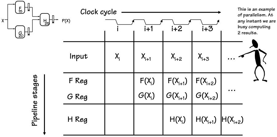
A pipeline diagram is just a depiction of what inputs are being processed during a given clock period. The results associated with a particular set of input data move *diagonally* through the diagram, progressing through one pipeline stage on each clock cycle.
