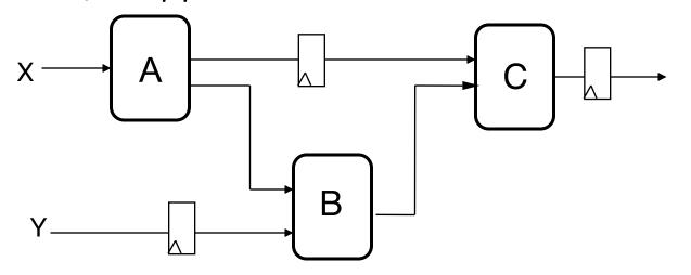
For what value of K is the following circuit a K-Pipeline? ANS: \_\_\_\_\_
