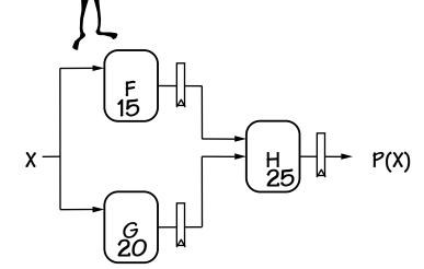
Now F & G can be working on input  $X_{i+1}$ while H is performing its computation on  $X_i$ . We've created a 2-stage *pipeline* : if we have a valid input X during clock cycle j, P(X) is valid during clock j+2.
