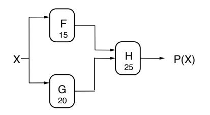
For combinational logic: latency =  $t_{PD}$ , throughput =  $1/t_{PD}$ . We can't get the answer faster, but are we making effective use of our hardware at all times?
