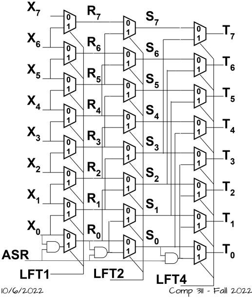
If we connect our "shift-left-two" shifter to the output of our "shift-left-one" we can shift by 0, 1, 2, or 3 bits.
