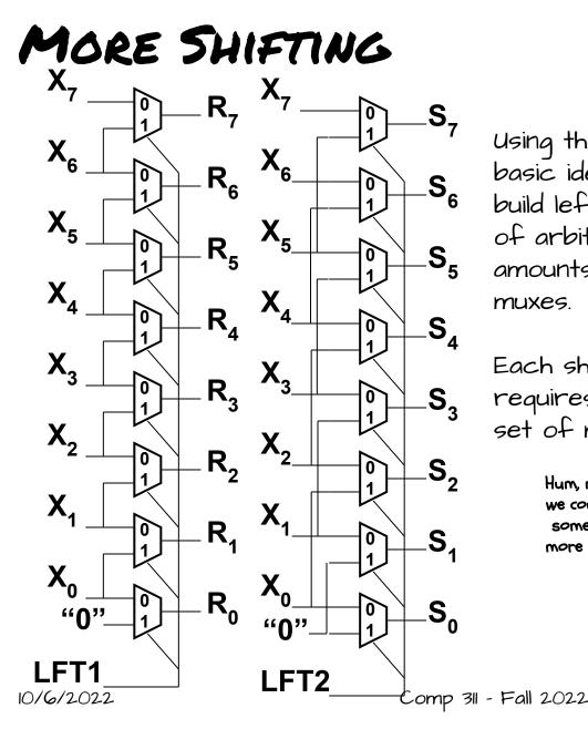
Using the same basic idea we can build left shifters of arbitrary shift amounts using muxes.
